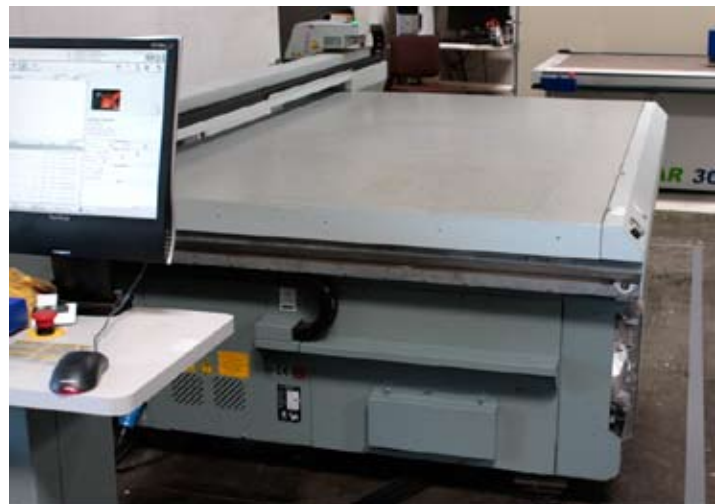
Flatbed UV Printer - 4'x 8' up to 1.75" thick
