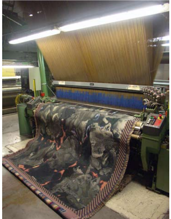
Bronco-X by Ed Moses being woven on an electronic Jacquard loom.
