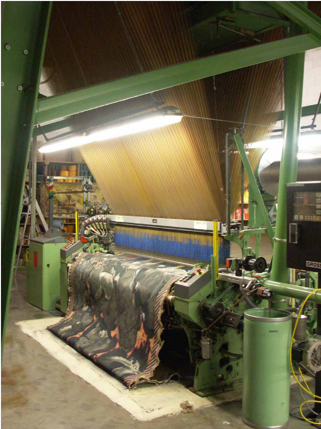
A 2002 tapestry by Ed Moses on the loom in Belgium; the 17,800 V-shaped threads above the loom are controlled by the dual Jacquard head. Photo by Donald Farnsworth.
