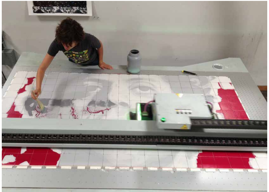
Master printer Tallulah Terryll paints a layer of underglaze on tiles for Subway Figures at Magnolia Editions while a large-scale flatbed printer lays down a layer of magenta acrylic ink to serve as a mask.
