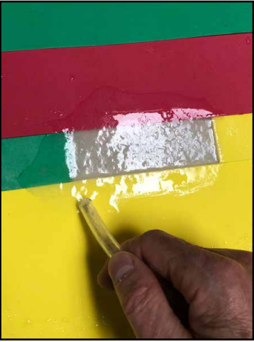
Using additional suction to remove excess furnish from foam masks
