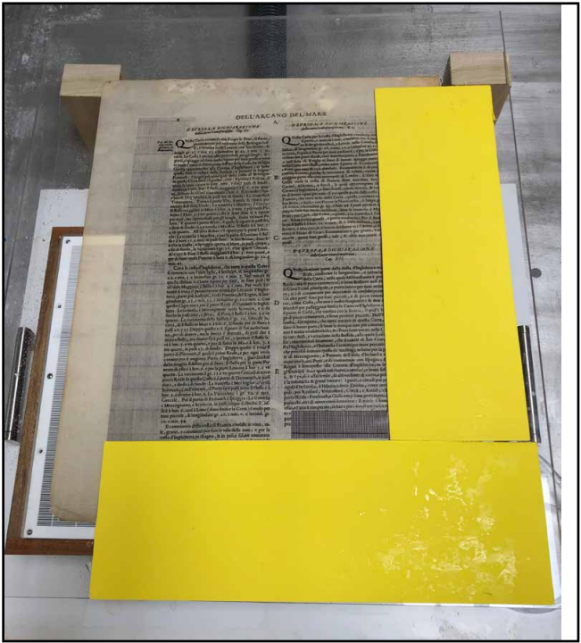
Partially masking a document that is larger than the leaf caster, supported by a clear Plexiglas platform
