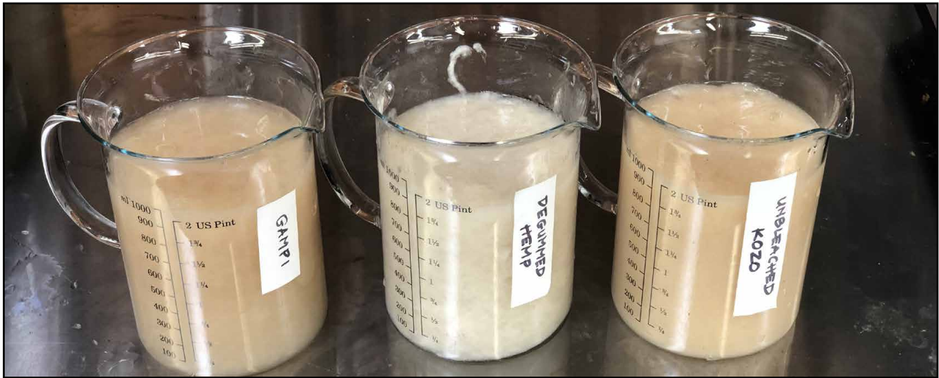
Three pulps blended and ready for mixing in the proper proportion of 68% gampi to 16% hemp and 17% kozo. I use beakers with handles as neri is very slippery – get a little bit on your hand and a beaker will slip right out.
