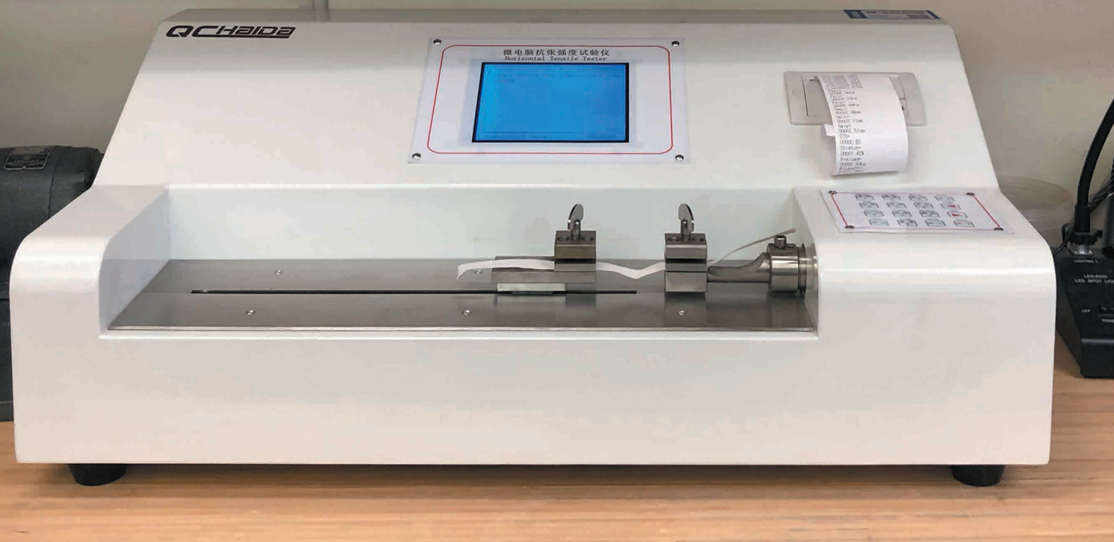
Haida HD-1512 Horizontal Tensile Tester at Magnolia's paper studio
