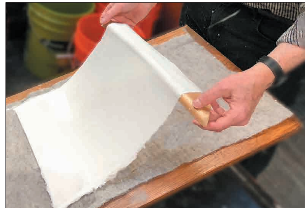
After pressing, lift sheet using a slice, separating it from the felt; then lay it right back down on the same damp felt and let it air dry – for multiple sheets, use rack as seen on opposite page
