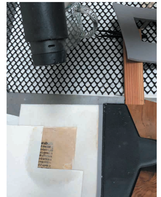
Mask removed; slow drying while under vacuum
