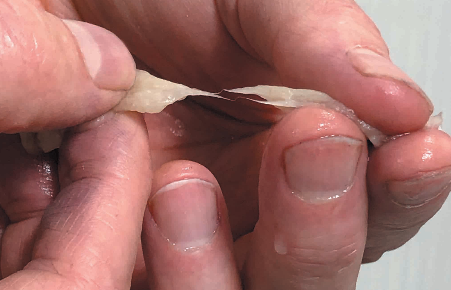
Handling a piece of freeze-dried furnish after moistening: note hydrogen bonds have not formed, making the fibers easy to pull apart
