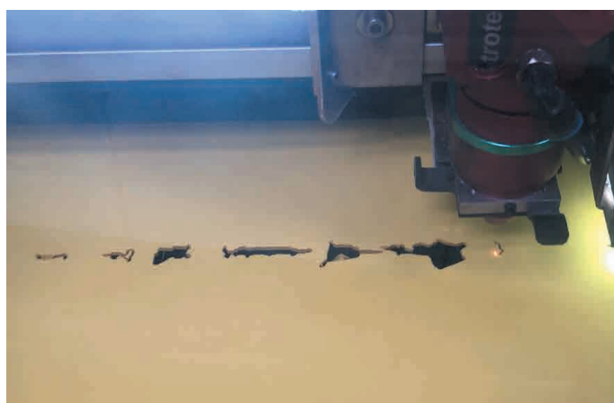
Laser cutting a foam mask to form the infill shapes
