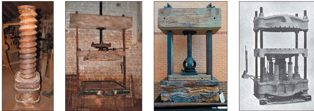
Dewatering technology's transition from wood screw presses to wood and steel and finally, to hydraulic presses
