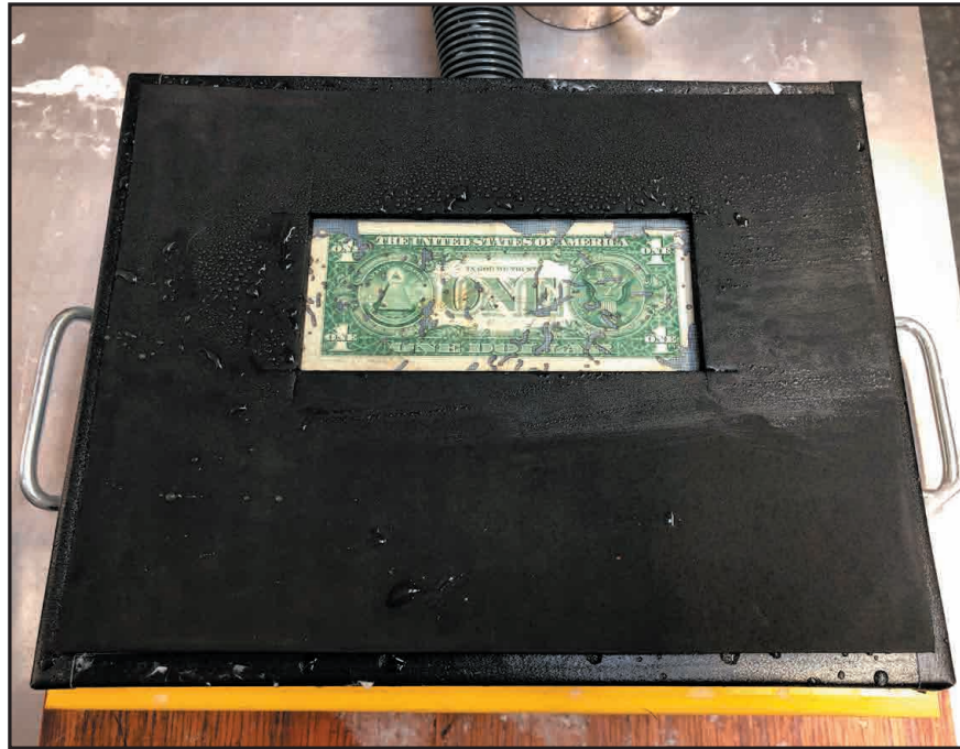
Worm-eaten dollar moistened and relaxed on 86 mesh polyester screen with cut foam mask – viewing side down
