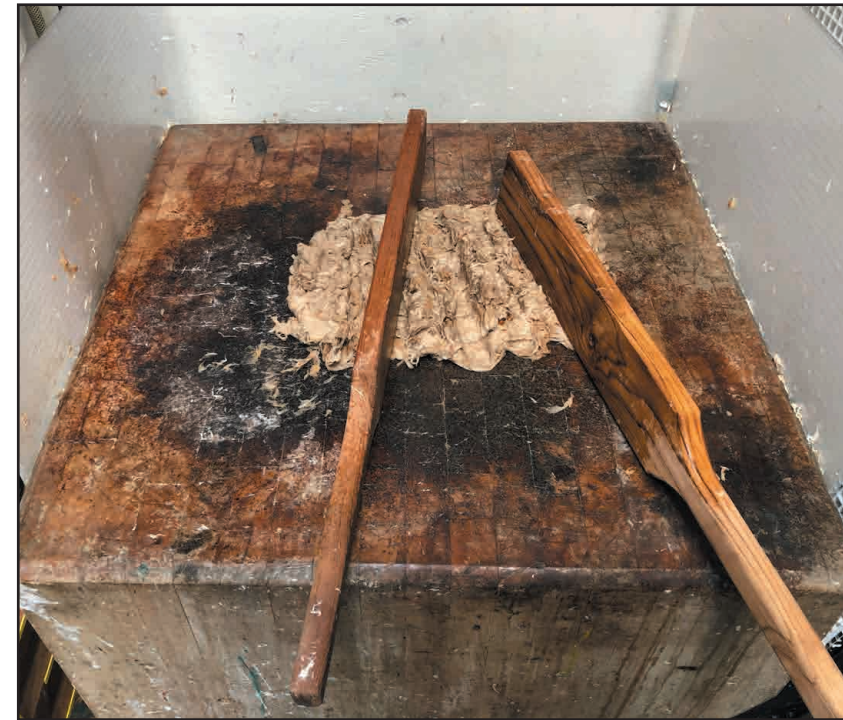
Harvested, stripped, soaked, scraped, cooked, and hand-beaten kozo. Once freeze dried, if kept dry, it can be stored for decades. When re-moistened, it's right where you left off – ready for more beating or simply to be stirred into a bucket of water to make furnish.
