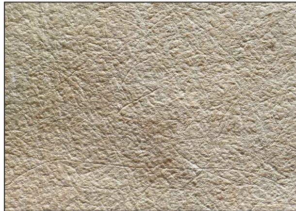
Air dried sheet (dried unconstrained for maximum surface texture)
