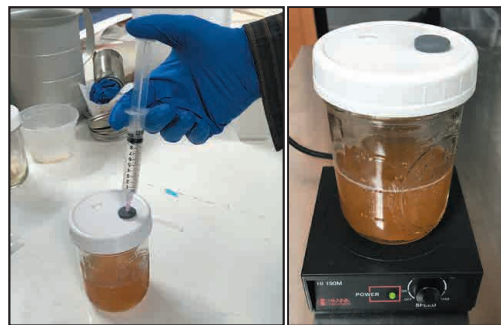
Inoculating sterilized 3% solution of malt and dextrose and stirred for 48 hours
