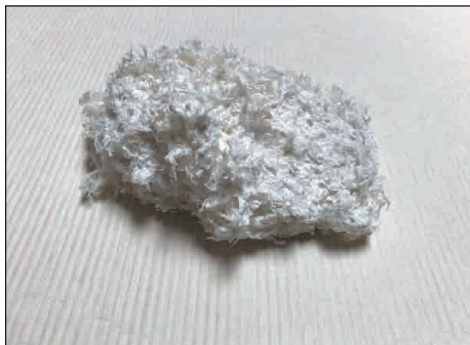
Cheney rag half-stuff (staple fiber) on top of a sheet of Celesa flax half-stuff
