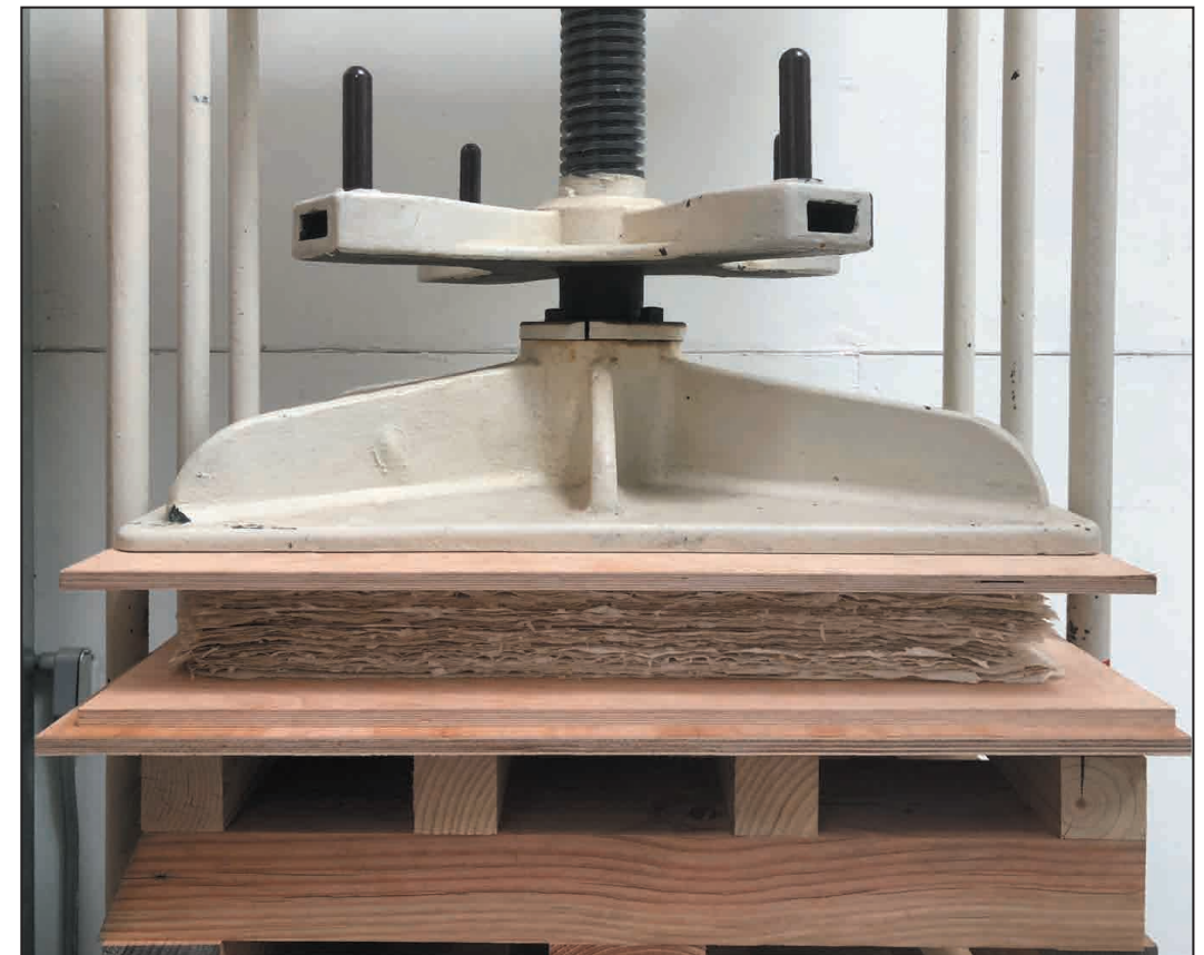
Curing paper under pressure in a standing press
