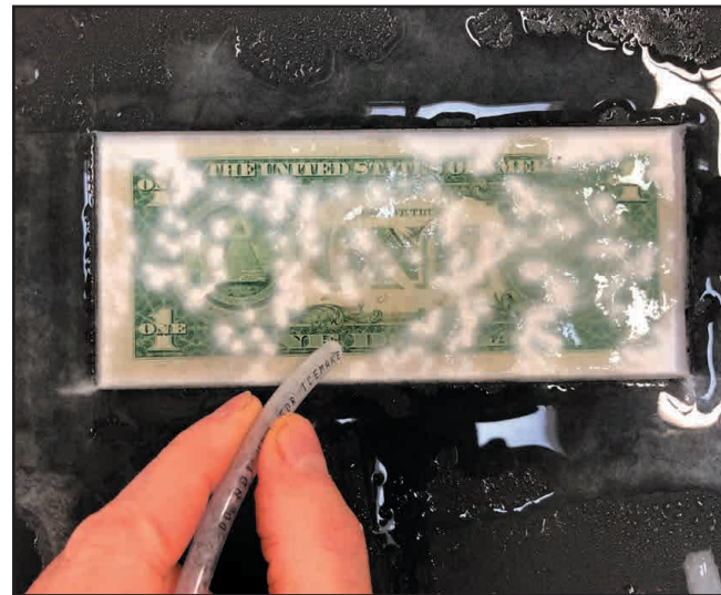
Using the ¼ inch vinyl tube connected to the suction of the leaf caster box to carefully remove excess furnish in the non-casting areas
