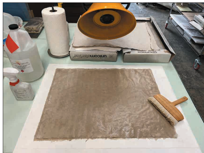
Sheets of paper moistened with water and alcohol and mizubake (water brush)
