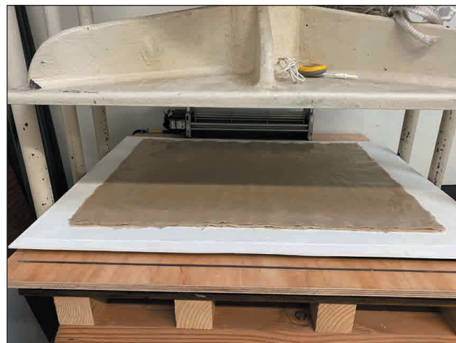
Sheets of paper moistened paper being loaded into a stack dryer. The cross-flow fan can be seen at far side of press.
