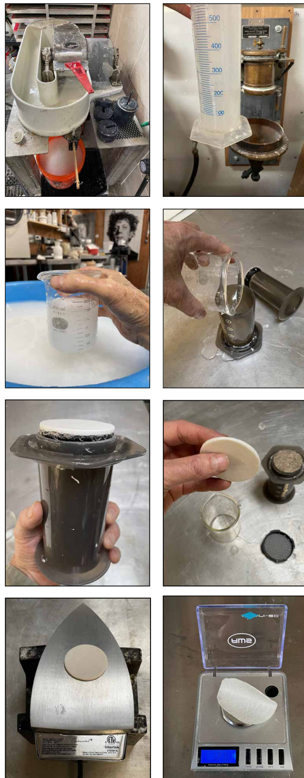
From left to right top to bottom: Beating, Testing Freeness, taking sample from vat, Pouring sample into Arrow Press, Paper Puck at tip of Arrow Press after pressing, The paper puck, Drying puck on inverted iron, weighing puck.
