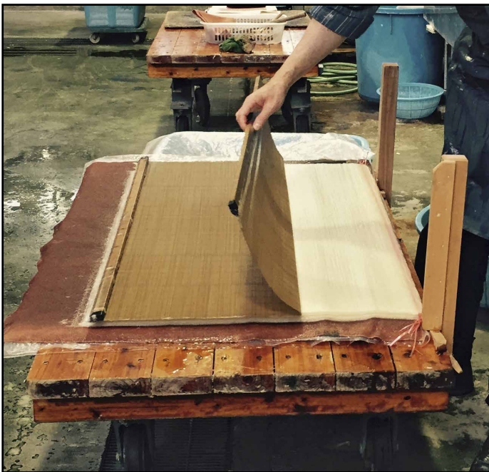
The hiss and snap of the su being lifted as a washi is couched
